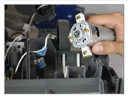
• Take the motor out and away from the motorized floor brush compartment by hand.
