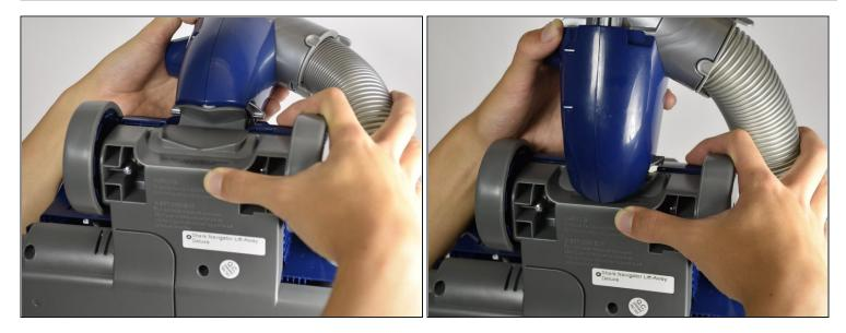
• Move the blue fulcrum connecting the bottom and the main body of the vacuum cleaner back and forth to loosen up crevice between the two halves of the roller brush enclosure.
