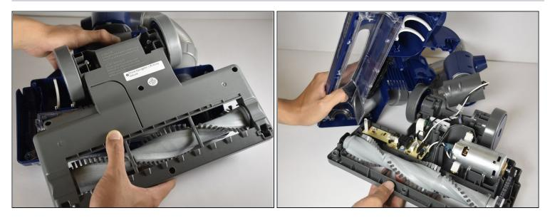
• Lift the grey frame off the bottom of the vacuum cleaner with your hands and place it on a flat surface.
