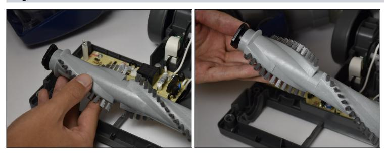
• Remove the roller brush from the plastic frame using your hands by lifting it away.
