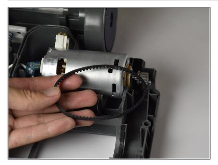
• Remove the roller brush belt with your hands by sliding it of the end of the motor.
