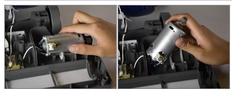
• Lift the roller brush motor up and away from its half-cylindrical holder with your hand.
