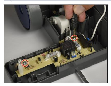
• Locate and remove the two 10mm screws on the motherboard with the PH1 screwdriver.
