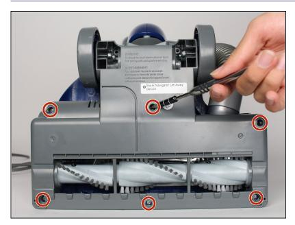
• Remove the six 15mm screws using the PH1 screwdriver.
