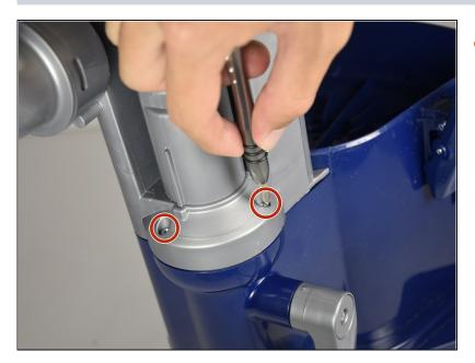
Remove the two 15mm screws with the PH1 screwdriver located on the bottom side of grey plastic body from which the handle was removed.
