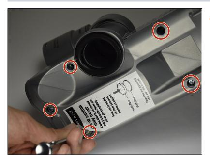
Locate and remove the five 15mm screws with a PH1 screwdriver.
