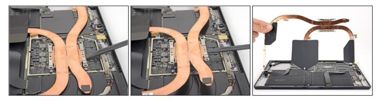
Use the flat end of a spudger to gently pry the heat sink straight up and off of the CPU.
