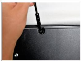
Remove the 36 silver 10mm J head screws with a J1 screwdriver from the back panel.
