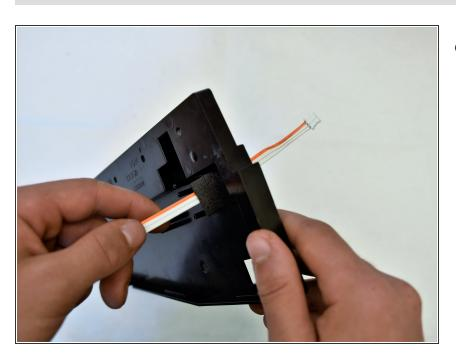
Run the white and orange cable through the innermost side panel and pull out
