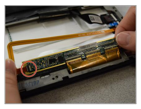
Disconnect the ribbon wire from the LCD connector by gently pulling it.
