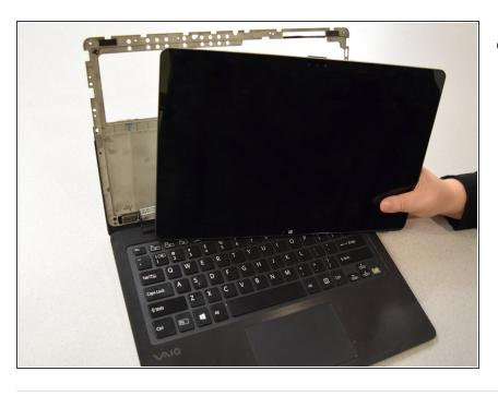
The screen can now be removed and replaced.
