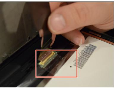
Gently pull up on the tape at the bottom of the ribbon to unplug the screen connector from the screen.
