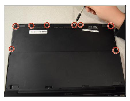
Looking at the back of the screen, remove all 8 screws using a Phillips #0
