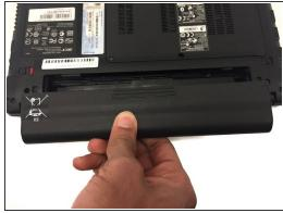
Hold the battery release button, and pull the battery out of the laptop.
