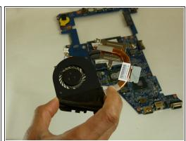
Carefully remove the fan from the motherboard by detaching the plastic insert as seen in the pictures
