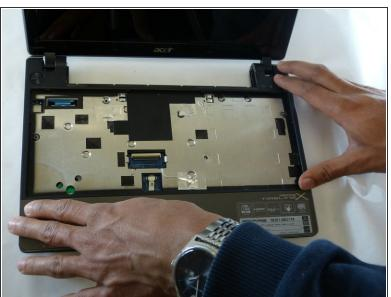
Use a Phillips #0 screwdriver to remove the 4 screws from the motherboard shield.
