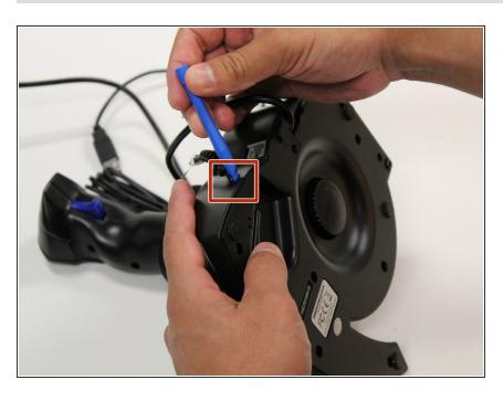
Insert opening tool or finger into the divet located beneath the USB port.
