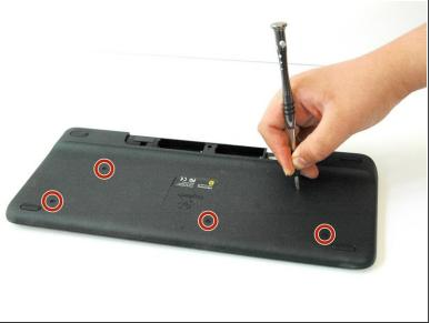
Unscrew all five 4.0 mm screws, using Phillips #1 screwdriver.
