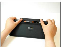
Press and slide up on the upper battery latch, using both thumbs.
