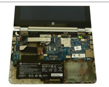
After the ribbon cables are disconnected, gently lift up the keyboard to disconnect it from the base of the laptop.
