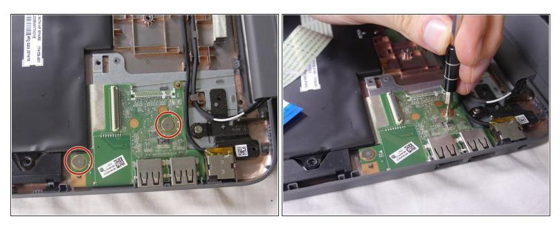
• Remove two 2mm screws from the I/O board using the Phillips PH00 screwdriver.
