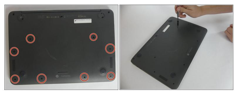
With the Phillips #00 screwdriver, remove the remaining eight 6mm screws. You will now have thirteen 6mm screws removed from the case.
