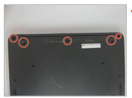
Remove the five 6mm screws located under the removed pads using Phillips #00 screwdriver.
