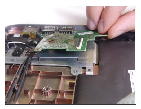
• Lift the I/O board out of the laptop case.
