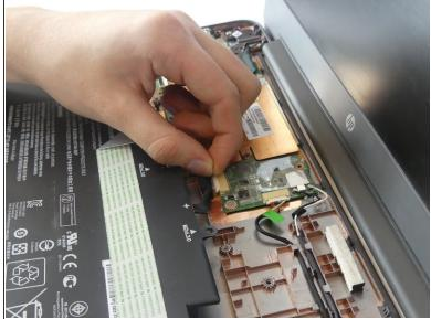
Unhook the battery's power connector from the motherboard.
