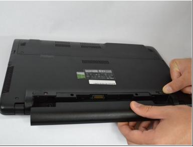
Push the left switch outward and push the battery upward at the same time.
