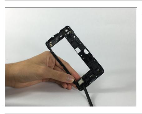
On the back panel, use a plastic spudger to remove the speaker.
