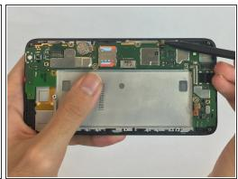
Using the spudger, pry open the zif connector, and remove the cable.
