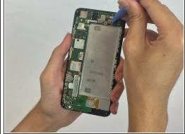
Use the plastic opening tools to remove all the remaining flat-top connectors
