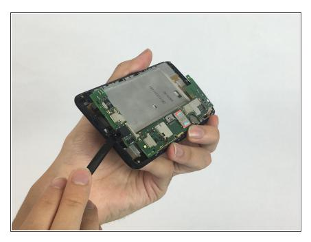
Using flat-side of spudger, remove the motherboard.
