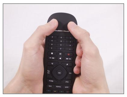
• Push the battery cover upward.
