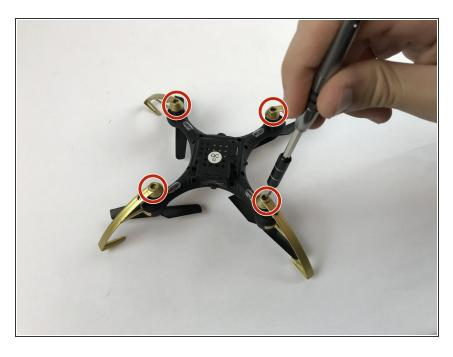
Unscrew the top four screws using a Phillips #0 screwdriver.
