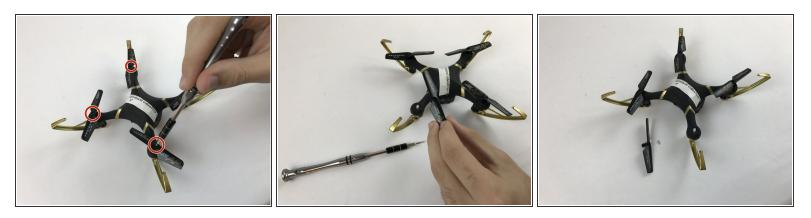
• Using #0 Philips head screwdriver, unscrew the four propellers.
