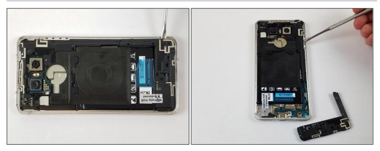
• With the screws removed, remove the lower frame components, followed by the upper mid-frame. Both components can be removed with a little prying.
