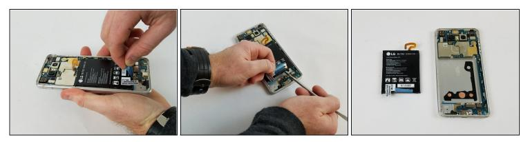
• Firmly pull the blue tab. Be careful not to bend the battery as you pull it away from the adhesive.
