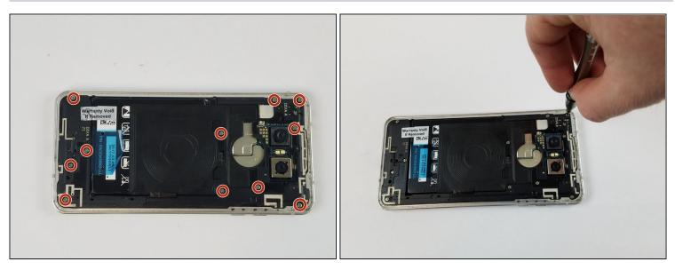
• Using a Philips 000 bit, remove 11 screws from the highlighted locations.
