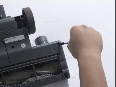
Remove the four 18mm screws located on the top corners and the bottom/middle of the vacuum head using a JIS 1 screwdriver.
