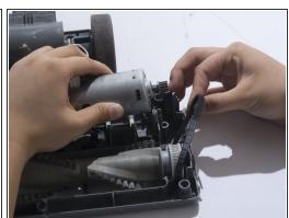
Remove the belt, found on the right hand side, from the motor gear.
