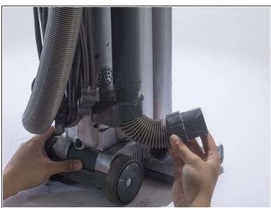
Detach the hose connected on the bottom of the vacuum by pulling it out of the casing.
