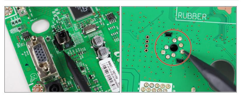
Desolder each of the indicated leads on the back of the motherboard.
