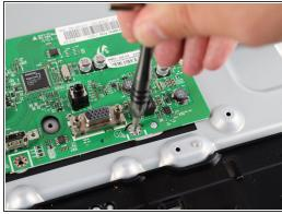
Remove each of the 5mm length screws attaching the motherboard to the body of the monitor using a #1 Phillips head screwdriver.
