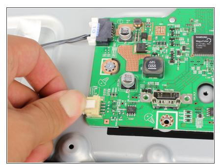
Remove the navigation button connector by pulling while holding down its thumb tab.
