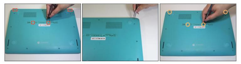
• Pry off the four rubber bumpers, located at the top corners and center of the back panel, off with a pair of <u>tweezers</u>.
