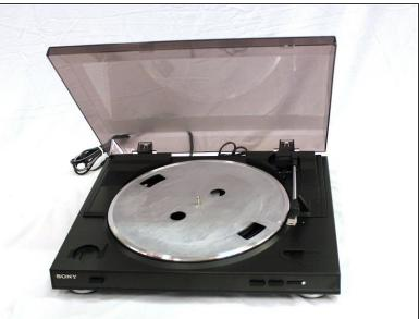
Lift the rubber mat, and put it to the side. It should be easy to remove, because it simply rests on a metal platter without anything securing it down.
