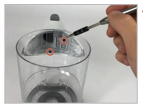
• Use a T8-Torque screwdriver to take out the two 26mm screws out.
