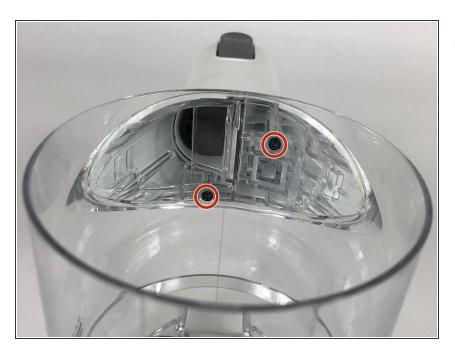
• Locate two screws at the back of the attachment holder.
