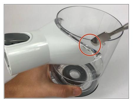
• Loosen the attachment holder by using a metal spudger.
