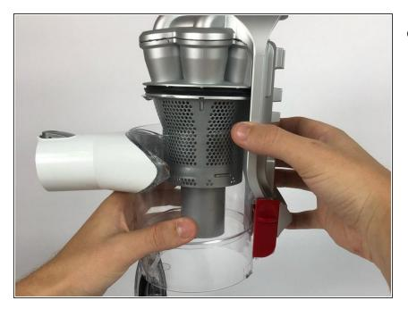
Push the red lever, pull the back up and away from the dust bin to separate them.
