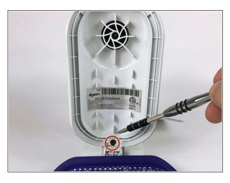
Locate and remove the 10mm
