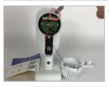
Use a flat spudger to loosen and remove the motor out of the vacuum.
