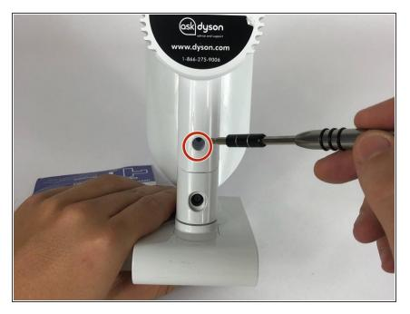
Take out the 10mm screw using a Phillips #1 screwdriver.
