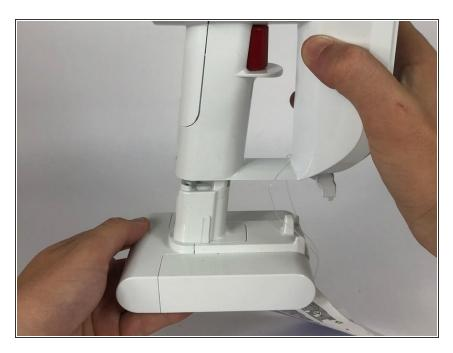
Pull the battery pack down and away from the main body and remove it from the device.
