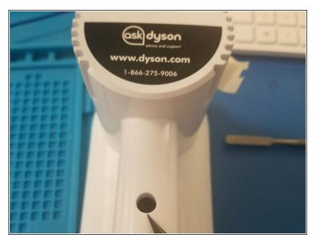
Locate and remove #000 25mm phillips screw on the reverse side of the vacuum
