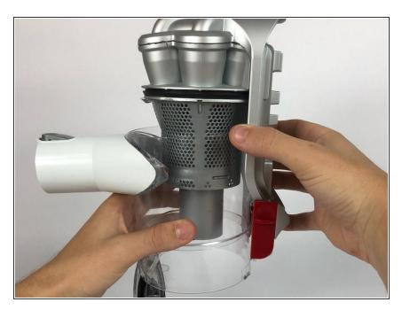
Push the red lever, pull the back up and away from the dust bin to separate them.
