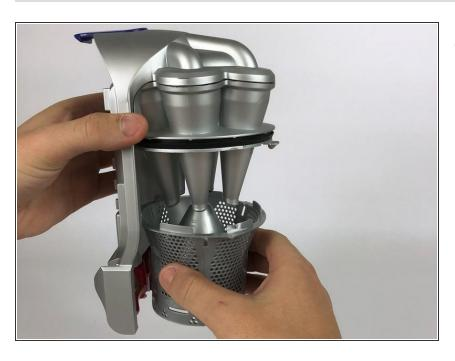
Remove the rest of the cyclone screen by pulling down.
