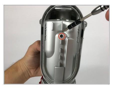
Use a T8-Torque screwdriver to remove the 18mm screw from the back of the Cyclone.
