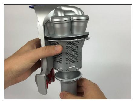
Remove the bottom of the cyclone screen by twisting it to the left and pulling down.
