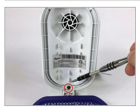
Locate and remove the 10mm
