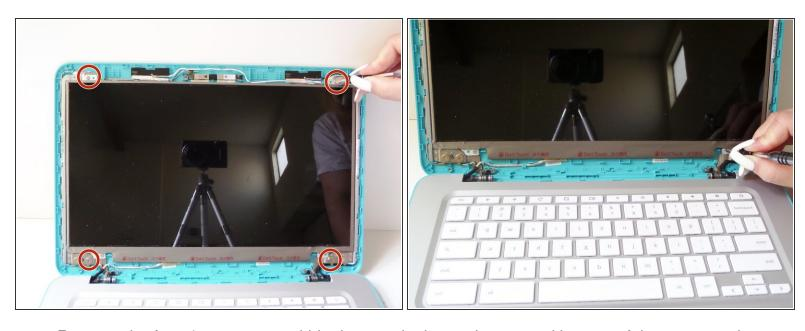
Remove the four 4mm screws within the metal tabs on the top and bottom of the screen using a Phillips Head 1 screwdriver.
