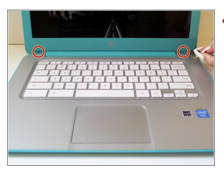
Remove both 4mm screws using a Phillips Head 1 screwdriver
