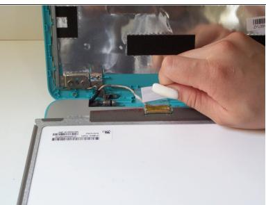
Peel off the barcode sticker to reveal the screen connector plug.
