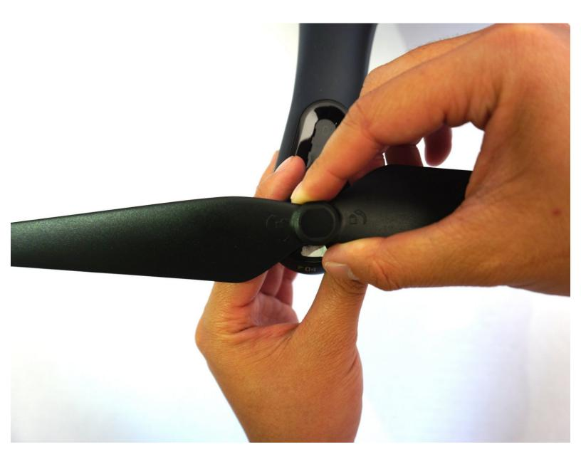
3DR Solo Propeller Disassembly
