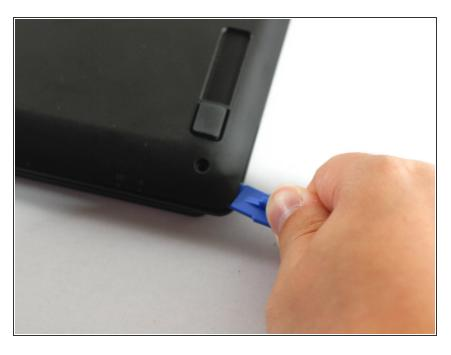
Using your prying tool, carefully remove the back panel.
