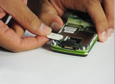
• The Sim card can simply be pulled out through the opening.
