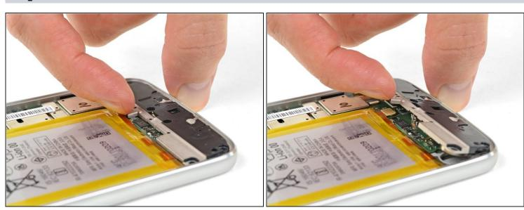
Pry up and remove the lower cover.
