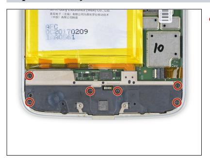
• Use a T3 Torx driver to remove the six 3.2 mm screws securing the lower cover.
