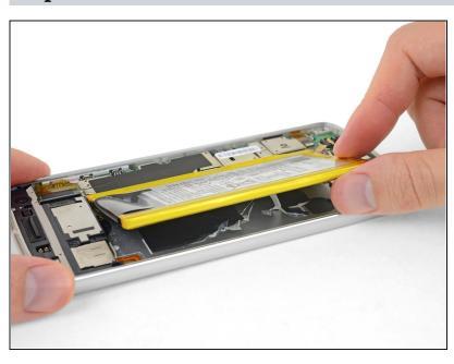
Continue pulling up the battery until all the adhesive releases from the rear case.
