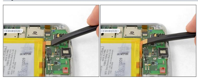
• Use a spudger to disconnect the battery by prying its connector straight up from the motherboard.
