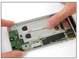
• Place <u>stretch-release adhesive strips</u> or several strips of thin double-sided adhesive tape, either from a <u>pre-cut adhesive card</u> or from a roll of <u>Tesa 61395</u>, into the battery well, and press them firmly into place.
