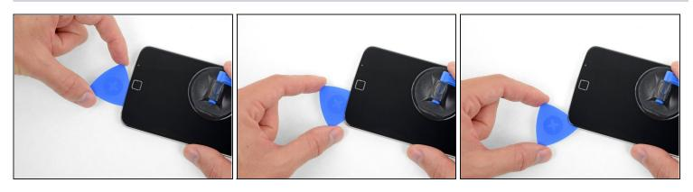
• Continue separating the glue underneath the rest of the lower bezel.
