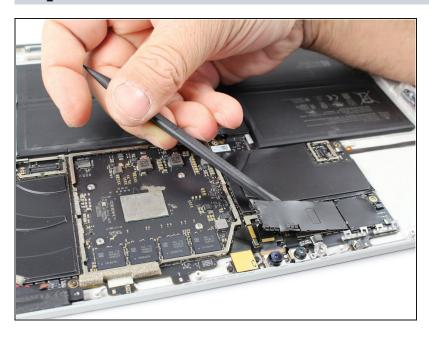
Pry off the metal cover covering the front and rear camera ribbon cable motherboard connections using a nylon spudger.
