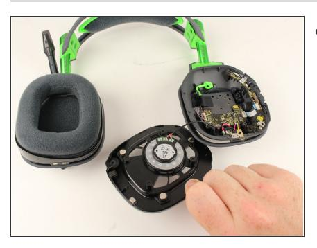
Lift the speaker module up off the device.
