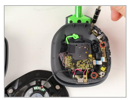
Remove the three 6mm PH1 screws.
