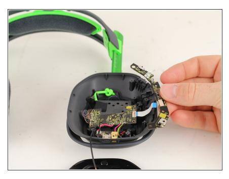
Dettach the thin circuit board from the ribbon with your hand by pulling the board and wire in different directions.
