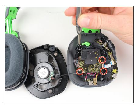
Remove the four 6 mm PH1 screws.
