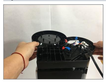
Unscrew and remove the heating plate layer. This will expose the internal workings of the machine.
