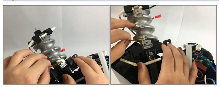
• Locate the coated wire that feeds into the side of the water heating element. Remove this wire.
