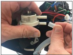
• Remove the tubes attached to the side of the water pump.
