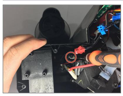
Unscrew and remove the remaining J1S1 screws that secure the water heating element to the interior of the device.
