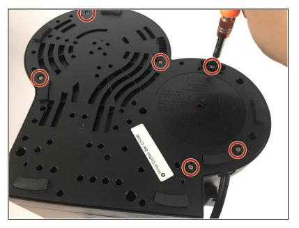
Unscrew the T-10 screws from the bottom cover of the machine, and remove that bottom cover.
