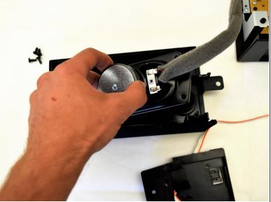
Grasp the speaker from the center and lift the speaker out of the panel.
