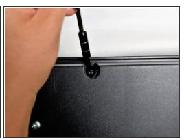
Remove the 36 silver 10mm J head screws with a J1 screwdriver from the back panel.
