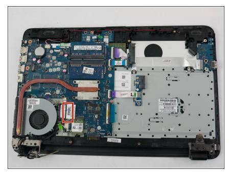
Disconnect the display ribbon cable from the motherboard.
