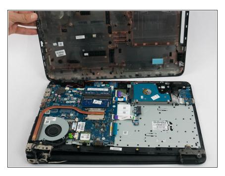
Lift off the bottom cover, exposing the motherboard and other components underneath.
