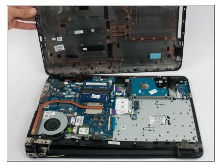
Lift off the bottom cover, exposing the motherboard and other components underneath.
