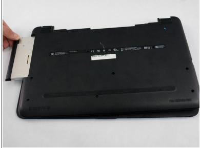
Remove the optical disk drive from the side of the laptop.
