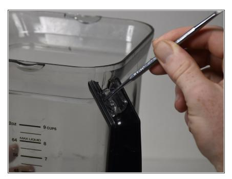
Unhook the latches from each side of the top portion of the handle with the metal spudger.
