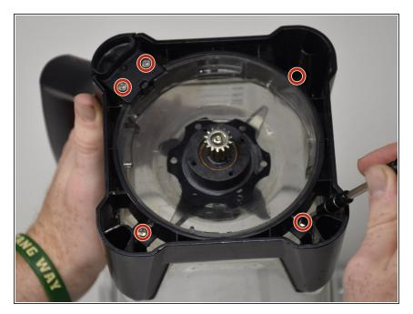
Remove five Phillips #2 9mm screws on the bottom of the blender.
