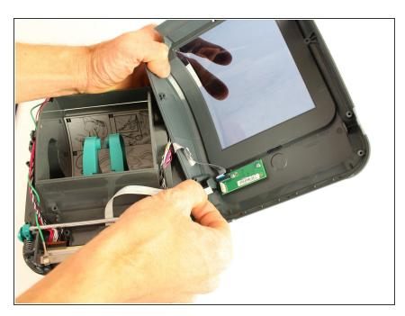
Carefully remove the ribbon cables from feed key.
