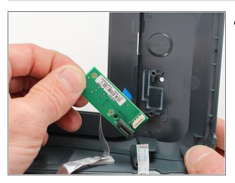
Lift and remove the feed key from the printer.
