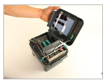
Close the printer and remove the top cover.
