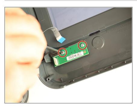
Remove the two P0 6mm screws securing the feed key.
