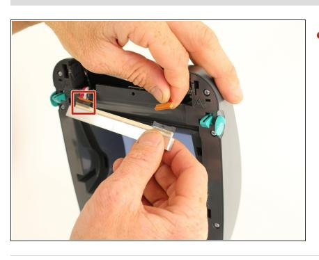
Disconnect the two (tan) harnesses located on opposite sides of the thermal head and remove the printhead.
