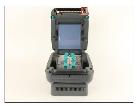
Locate a tab securing the printhead on the right hand side of the printer.
