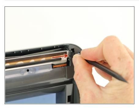
Push the tab to the right. The thermal head should release outward.
