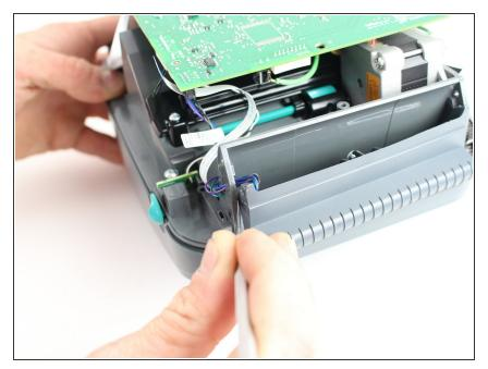
• Remove the peel and present system by utilizing a metal spudger.
