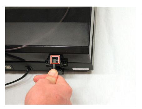
Use a flat head screw driver to apply pressure to the black square button on the right side.
