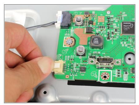
Remove the navigation button connector by pulling while holding down its thumb tab.
