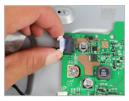
Remove the screen connector by gripping its sides and gently pulling while wiggling back and forth.
