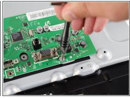
Remove each of the 5mm length screws attaching the motherboard to the body of the monitor using a #1 Phillips head screwdriver.
