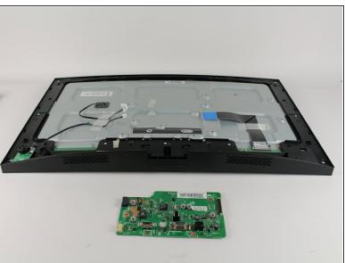
Using both hands, lift the board off of the monitor body by the motherboards base.
