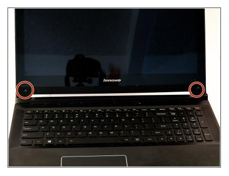
Remove the black plastic or rubber screw caps covering screws, located at the bottom of the screen
