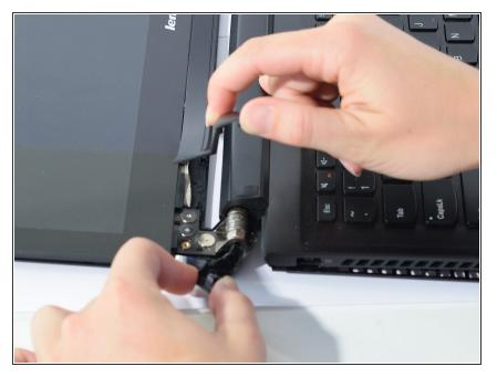
Pry apart plastic cover at the bottom of the screen from plastic hinge cover.
