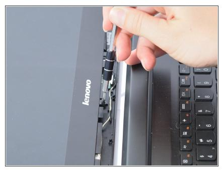
• Remove the (1) M2.5 x 2.5mm Black Phillips, Nylok coated screw located near the bottom center of the screen with the Phillips #1 screwdriver.
