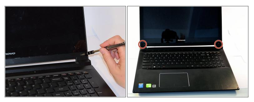
Remove the (2) M2.5 × 2.5 mm, Black Phillips Nylok coated screws with the Phillips #1 screwdriver, located on either side of the bottom of the screen.
