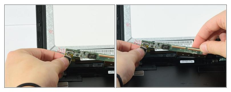
• Unplug the sensor from the sensor board near the bottom left of behind the screen.
