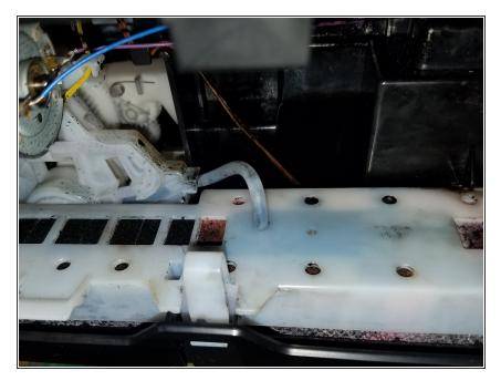
Connecting the ink TUBE to the newly cleaned/replaced ink pads.
