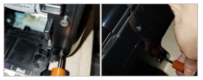
• THEN UNSCREW THE 2 VERTICAL SCREWS on the right side -- AND THEN the 2 vertical screws at the exact opposite side (THE BACK) of that same panel which encloses the right side of the printer. There are no other screws than those 4.
