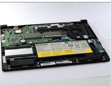
Gently lift the cover plate off the body of the laptop, ensuring that it does not pull on any components such as the USB ports.
