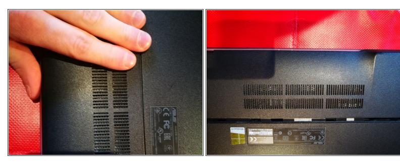
Remove the bar at the bottom of the laptop, by sliding it downwards.
