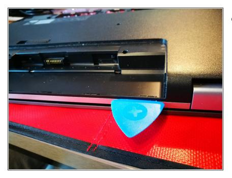
Use opening pick to create an opening at battery side. Try to open the battery side with opening pick only. Only when necessary use the spudger on this side.
